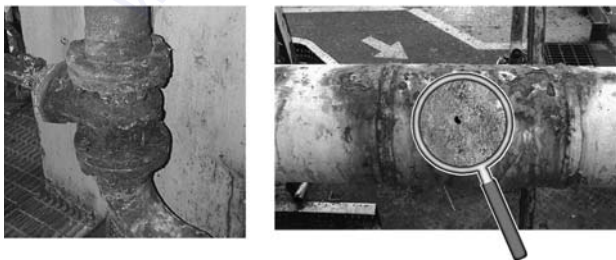
Figure 7.9 Corrosion under insulation (CUI)
