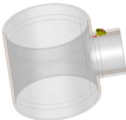
Figure 11-13 3D CAD image of nozzle with PA probe
