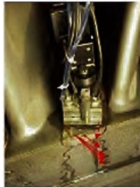
Figure 11-8 PAUT on steep section of turbine disc (21)
